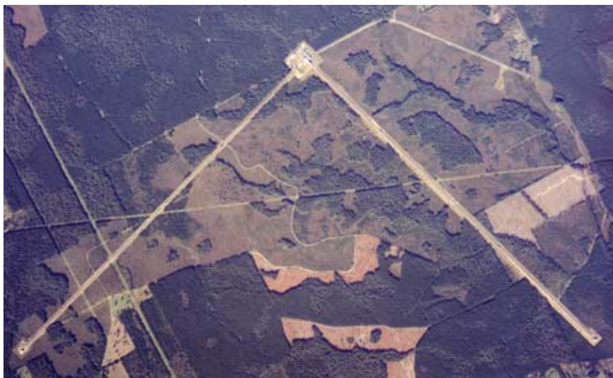
Figure 8. Aerial photograph of the LIGO facility in Livingston, Louisiana, reveals the grand scale of the apparatus with its 4-kilometer arms. (Courtesy of Rusty Gautreaux, Aero-Data.)
