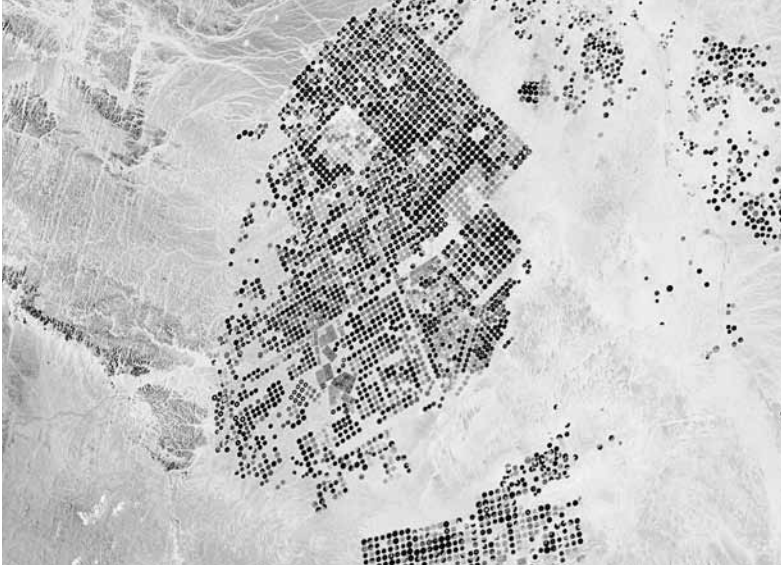
FIGURE 1.2. Pivot irrigation in the Wadi As-Sirhan Basin of Saudi Arabia, February 21, 2012. Fields in active use appear darker, fallow fields are lighter. Most are approximately one kilometer in diameter. As in Kansas, the water is pumped from underground. Credit: NASA Earth Observatory
