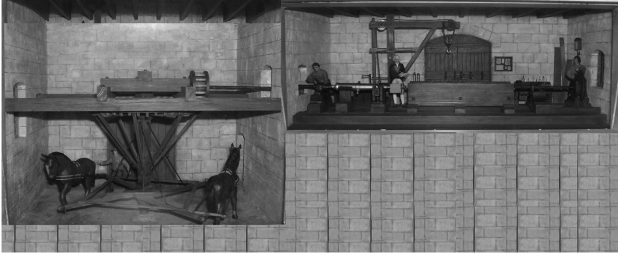
Fig. 9.1 A model of Rumford's cannon-boring experiment, 1789 (courtesy of the Rumford Historical Association, Woburn, MA).
