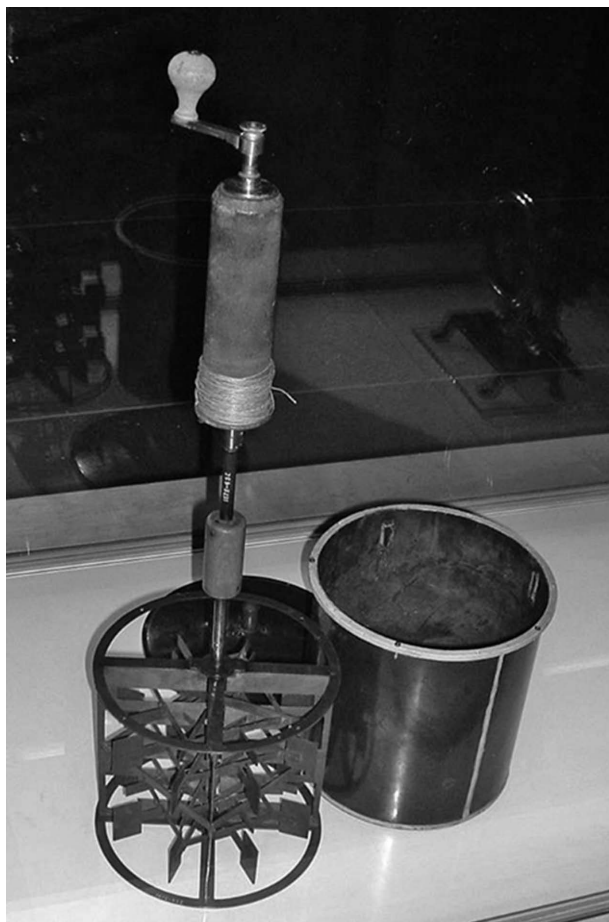
Fig. 14.2 Joule's paddle-wheel calorimeter, 1845 (Science Museum, London/SSPL).
