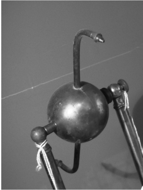
Fig. 2.1 A photograph of a reconstruction of Hero's steam toy (courtesy of the Museum of the History of Science, Oxford).
